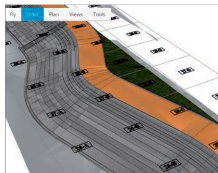
BIM model showing a grid overlay of the coastal scheme. Folders map to the grid, which makes it far easier and faster for users to locate the information that they need.
